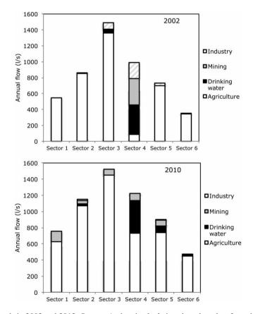
Fig. 7. Groundwater demands in 2002 and 2012. *Source:* Authors' calculations based on data from the study of DGA/DICTUC (2010).
